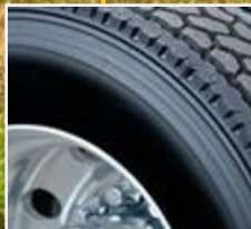
Bridgestone wide-based, low-rolling resistance fuel economy tires on the truck and trailer
