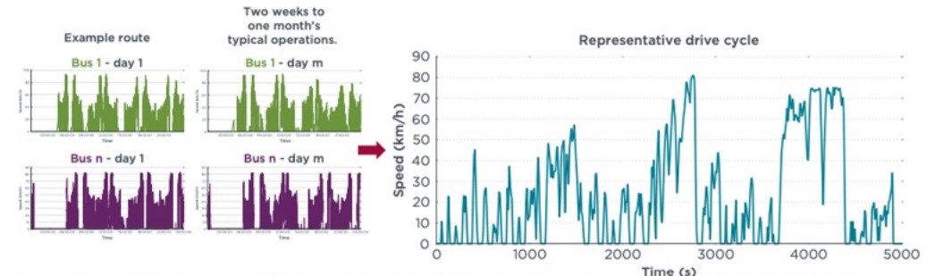
Illustration of a drive cycle developed for a route from real-world operational data. https://theicct.org/publications/zev-bus-fleets-dev-drive-cycles
